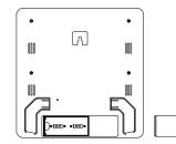
Insert finger or other solid object in the space at the bottom center of the battery compartment and lift up to remove the cover.
